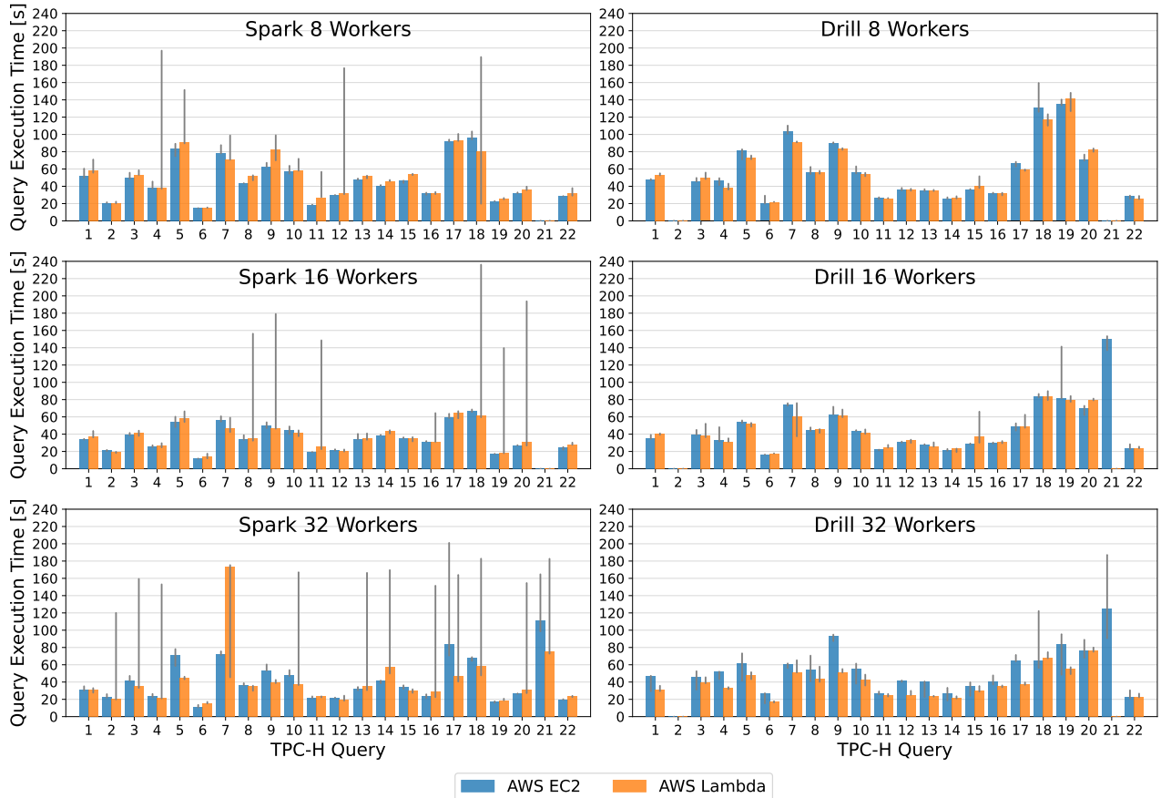
Figure 3: TPC-H (scale factor 100) query execution times for unmodified Apache Spark and Apache Drill running in AWS Lambda and AWS EC2. Median times of 3 executions of each query for each configuration, error bars are min. and max. times.
